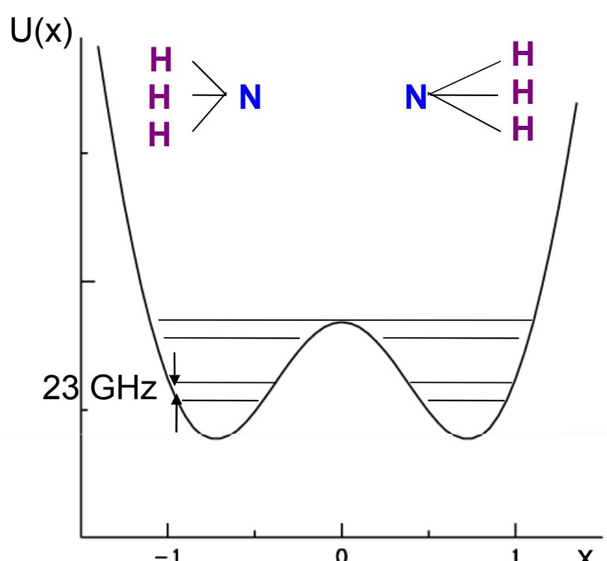
Double-well potential of the inversion vibrational mode of  $\text{NH}_3$
