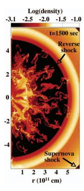
FIG. 7. (Color) Density distribution (log  $\rho[g/cm^3]$ ) 1500 s after core bounce. The supernova shock (outermost discontinuity) is located at  $r \approx 9 \times 10^{11}$  cm. A dense shell (visible as a whitish ring) has formed between the SN shock and reverse shock at  $r \sim 5 \times 10^{11}$  cm, with its outer boundary coinciding with the He/H interface. The fastest moving RT spikes have just reached the reverse shock. Adapted from Kifonidis *et al.*, 2003.
