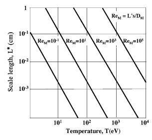
FIG. 28. Lines of constant magnetic Reynolds number  $Re_M$  = const for a fully stripped carbon plasma as a function of the characteristic length scale and temperature. Adapted from Ryutov *et al.*, 2001.
