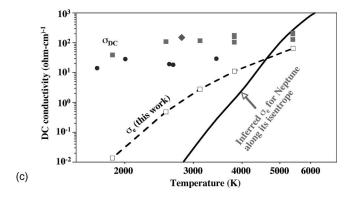
FIG. 36. The high-pressure properties of water are probed with strong shock experiments. (a) Plot of the measured EOS of water along the principle Hugoniot, at pressures up to ~1000 GPa. (b) Measurements of the reflectivity of shocked water vs shock velocity and shock pressure. (c) Analysis of the decomposition of the dc conductivity of water at high pressure along the isentrope appropriate for the interior of Nepture. Adapted from Celliers *et al.*, 2004.
