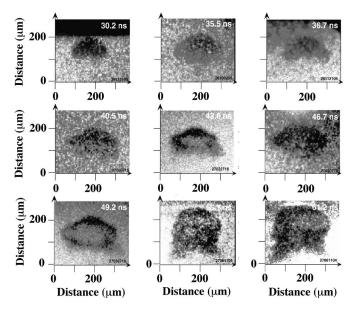
FIG. 16. Late-time evolution of the Cu sphere (scaled cloud) shock-cloud experiment, done on the Nova laser (Klein *et al.*, 2003). The experimental images span 30.2–61.2 ns, and show the evolution from the early-time aftermath of shock compression (30–40 ns) to the formation of vortex rings (42–49 ns), through the initial stages in the transition to turbulence (55–61 ns). Adapted from Klein *et al.*, 2003.
