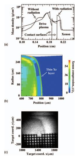
FIG. 20. (Color) Formation of a collapsed layer in dense Xe gas. (a) Density profiles calculated with the HAYDES code for the case with radiation (solid line) and no radiation (dashed line). Adapted from Reighard *et al.*, 2006. (b) Simulations using FCI2, of the 2D geometry, with the finite radius of the shock tube taken into account. (c) Radiographic image showing remarkable agreement with 2D simulations. Adapted from Reighard *et al.*, 2006.
