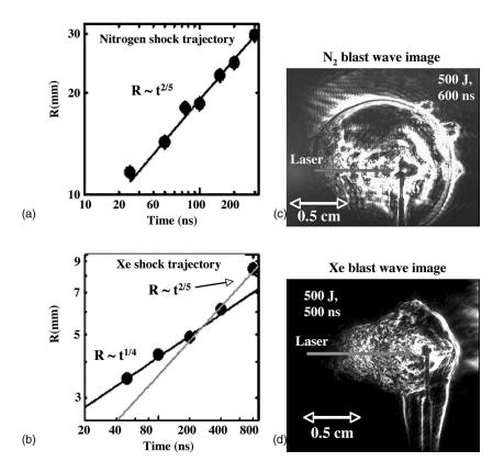
FIG. 22. Blast waves in nitrogen and xenon. Measured shock trajectories for (a) nitrogen and (b) xenon. Measured structure by dark-field imaging of the blast wave for 500-J energy input for (c) nitrogen and (d) xenon. Adapted from Edens et al., 2004.
