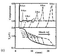
FIG. 23. The emergence of a second shock driven by the ionized precursor in strongly shocked Xe. (a) Schlieren image at t=150 ns and (b) at t=4  $\mu$ s. (c) The corresponding spherically symmetrical modeling. Adapted from Hansen *et al.*, 2005.
